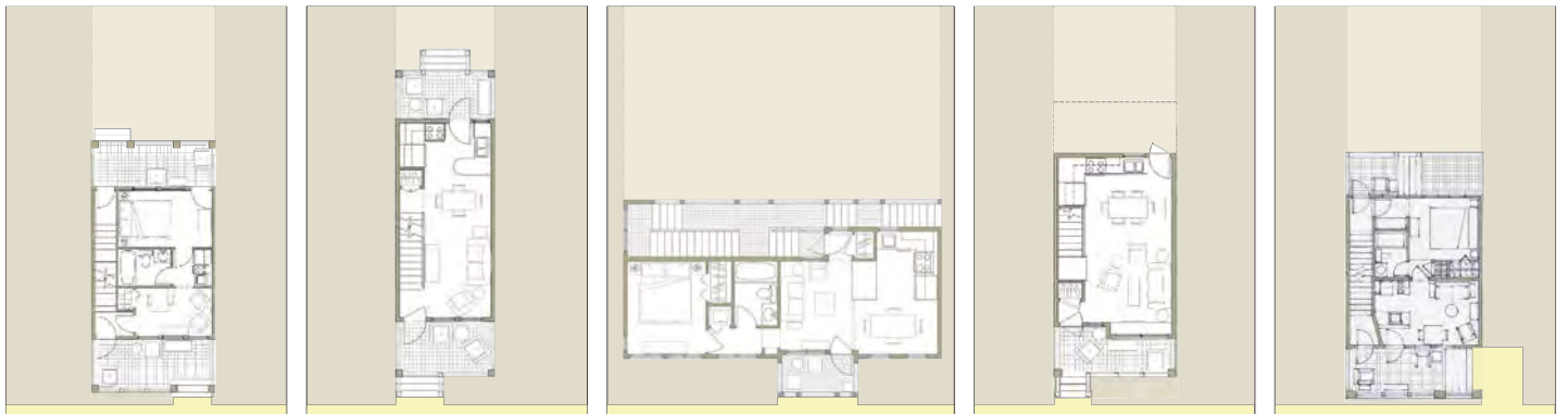
17x29 FLAT: 302 SF 12x25 TH: 715 SF 37x12 FLAT: 490 SF 15x22 TH: 790 SF 19x29 TH: 1,075 SF
