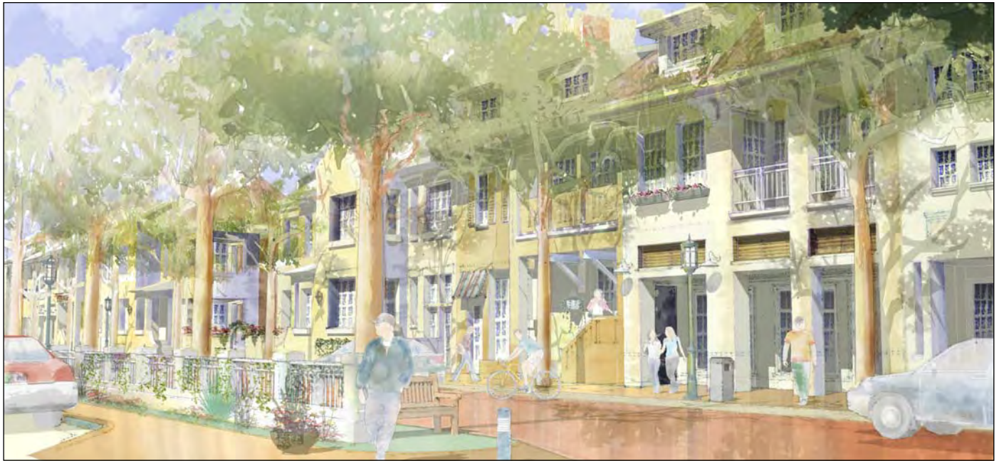
Small and moderate sized buildings can be arranged along a street front with considerable variety in height and width, so long as they are all the same (or complementary) building types. In this example, the buildings are rear yard (zero front and side setbacks), mixed use, pitched roof (with the eave and ridge parallel to the street), and designed with a shopfront/awning frontage type.
