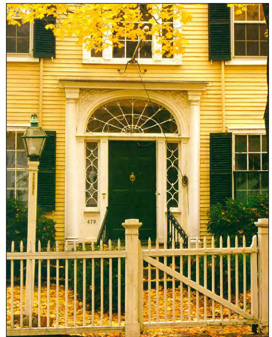
Figure 1. This "Porch and Fence" Frontage places the front building facade fifteen feet back from the street front line.
