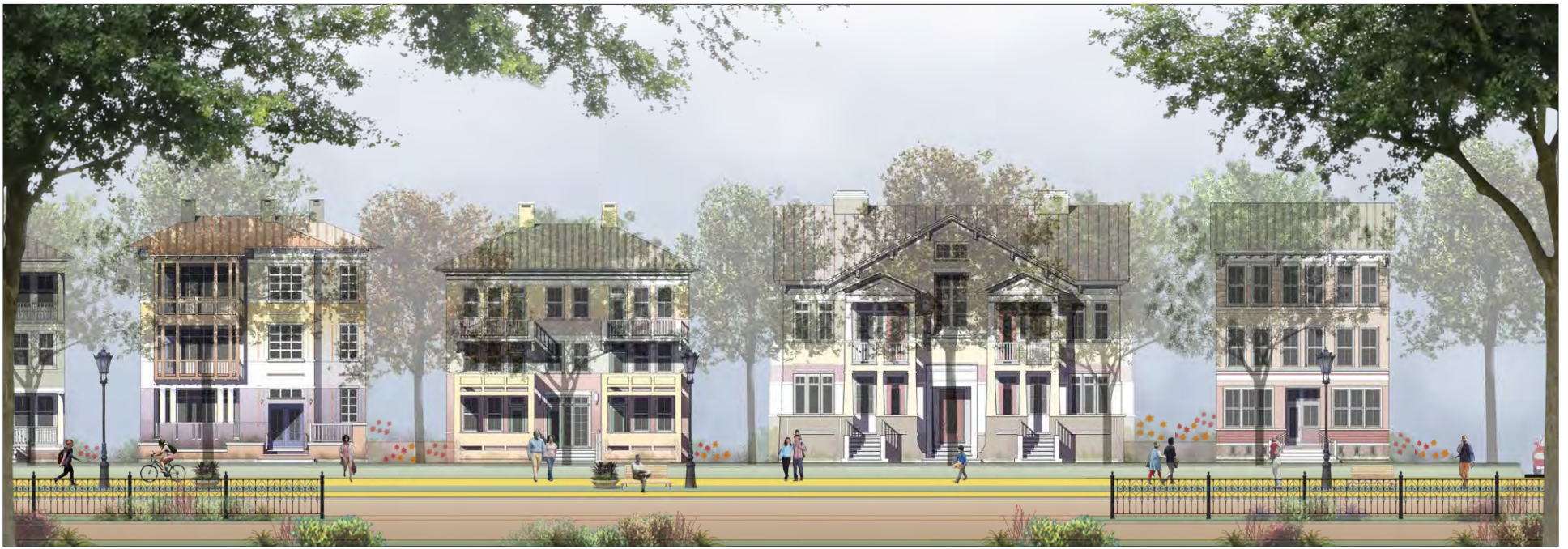
NEIGHBORHOOD GENERAL (T4.0 ZONE) STACKED UNITS/2-3 STORY SMALL-MODERATE BLOCK 4-6 UNIT FRONTAGE:PORCH AND STOOP
